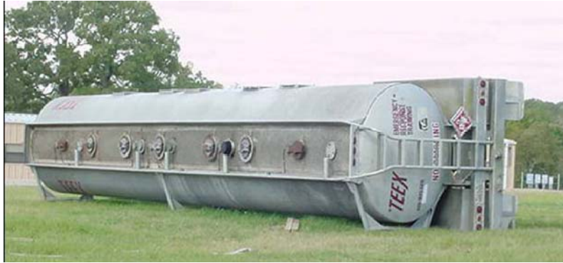
Figure 3.2: Overturned MC-306/DOT-406 Cargo Tank
